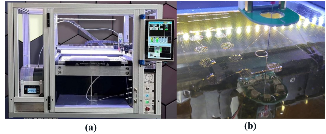
Figure 2: 3D printer system for sensor fabrication. (a) A commercial 3D printer from Hyrel 3D. (b) An image of the printer in operation.
