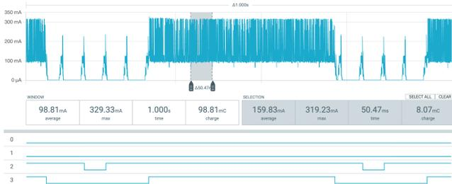
**Figure 5. Current trace that includes starting and stopping the Wi-Fi radio via BLE and transmitting data via Wi-Fi.**
