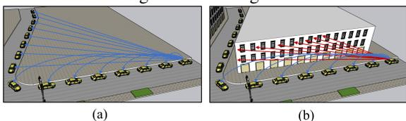
Figure 3: PMs around an intersection having (a) LOS communication with the PL due to no obstruction and (b) NLOS communication with PL due to obstruction by a building at the corner
