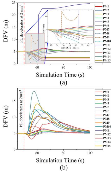
Figure 6: Comparison of DFV among PMs during PL deceleration at  $2m/s^2$ , for (a) CACC, and (b) AoI-aware CACC-based platoon of length 16
