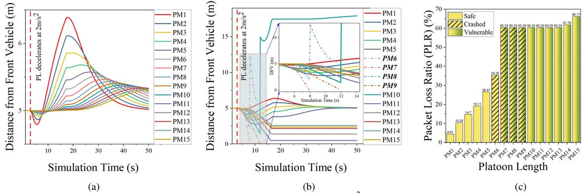
Figure 2: Comparison of DFV among platoon members when the leader decelerates at  $2\text{ m/s}^2$  under (a) LOS communication with PL, (b) NLOS communication with PL, and (c) the packet loss encountered by each PM on PL broadcast under NLOS communication
