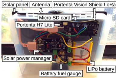
Figure 6. Testbed device and deployment
