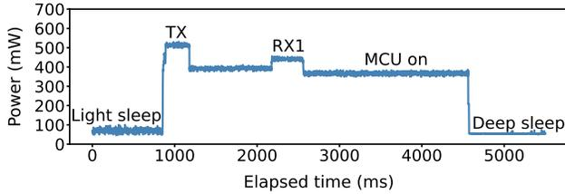
Figure 10. Power consumption profile of testbed device
