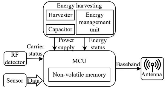
Figure 1: Overview of system architecture.
