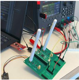
(a) Backscatter tag, carrier generator, and digital power supply.
