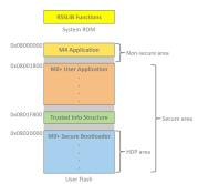
Figure 1. Flash partition and applied secure areas.
