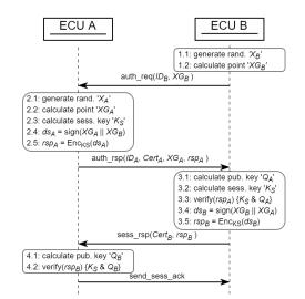
Figure 2. STS protocol based on the implicit certificates.
