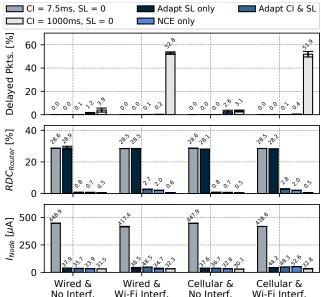
No Interf. Wi-Fi Interf. No Interf. Wi-Fi Interf. Figure 7. Performance of fixed and adaptive node configurations for sustaining  $\hat{t}_{TX_{MAX}} = 1000 \, ms$  on transmitting packets with a length of 128 bytes to a cloud server.
