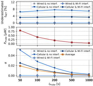
Figure 5. Percentage of underestimated  $t_{NET}$  values (top), power consumption  $P_{Probe}$  (middle), and cost  $\alpha$  (bottom) for different  $I_{Probe}$  values in four different environments.
