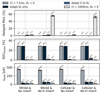
No Interf. Wi-Fi Interf. No Interf. Wi-Fi Interf. Figure 8. Performance of fixed and adaptive node configurations for sustaining  $\hat{t}_{RX_{MAX}}=1000\,ms$  on receiving packets with a length of 128 bytes from a cloud server.
