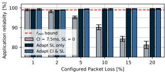
Figure 6. Measured end-to-end application reliability for different node configurations and configured packet loss.
