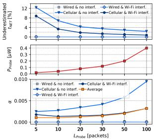
Figure 4. Percentage of underestimated  $t_{NET}$  values (top), power consumption  $P_{Probe}$  (middle), and cost  $\alpha$  (bottom) for different  $L_{Probe}$  values in four different environments.
