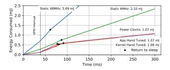
Figure 6: Cumulative energy of the *Groundwater Pollutants* application using five clock policies. All 3 dynamic policies perform within 1% of one another, while consuming 54-55% less energy than the best static clock choice over just a 300ms period. The savings come from no static clock choice being able to satisfy all device requirements *and* achieve lowest-power operation while waiting for a GPIO interrupt.
