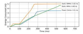
Figure 8: Cumulative energy of the multiple application example when the applications execute sequentially. Power Clocks consumes 25% less energy than the best static clock.
