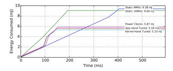
Figure 9: Cumulative energy of the *Audio Classifier* application with flash instead of radio for the K66. Power Clocks consumes 35% less than the best static clock. Power Clocks uses more energy than hand-tuned since it waits for a 10ms time quanta before switching clocks during compute, and has an extra transition to/from the low-energy clock at the end.
