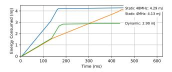
Figure 1: Cumulative energy used over time by an example sense-process-send application. Optimal dynamic clock management provides 32% energy savings over the best static alternative.
