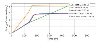
Figure 3: Cumulative energy of the *Audio Classifier* application using five clock policies. Power clocks is within 3% of the hand tuned in-kernel policy and consumes 27% less energy than the best static clock choice. Power Clocks performs worse than hand-tuned clock choices because the computation in the GPIO interrupt handler is much less efficient with a 115 kHz clock than with a 1MHz or 4MHz clock.
