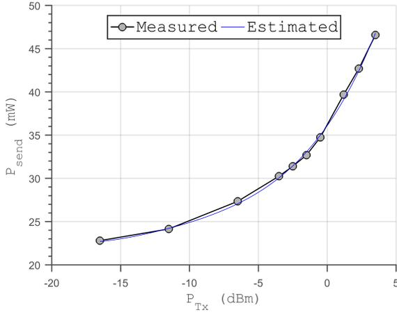
**Figure 3.** Power consumption as function of the  $P_{Tx}$ .
