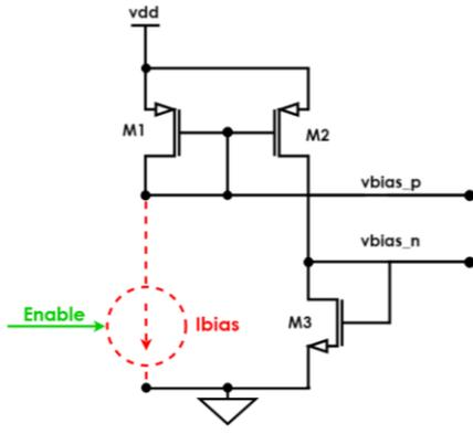
Figure 8. Bias generation circuit. In the simulations shown in section IV, is considered an ideal current source.
