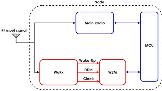
Fig. 5. WSN node with a WuRx including the baseband logic proposed in this paper and the WuRx to MCU interface (W2M).
