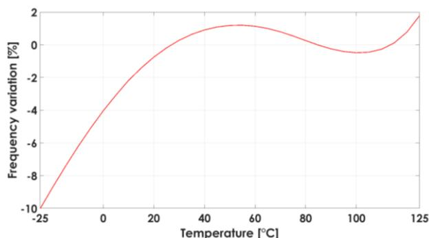
Fig. 12. Clock frequency variation with temperature.
