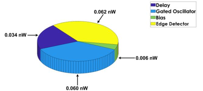
Fig. 10. Power consumption of the CDR during phase 1. CDR overall power consumption during phase 1 is  $P_{ph1} = 0.162$  nW.
