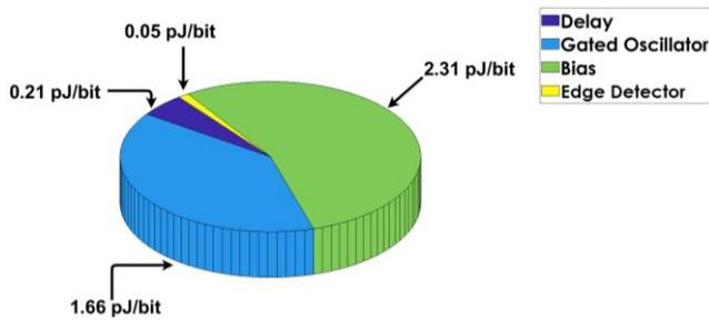
Fig. 11. Energy/bit consumption of the CDR during phase 2. At 1-kbps data rate the CDR overall power consumption is  $P_{ph2} = 4.23$  nW. CDR blocks contribution to  $P_{ph2}$  are:  $P_{ph2,Delay} = 0.21$  nW,  $P_{ph2,Gated\ Oscillator} = 1.66$  nW,  $P_{ph2,Bias} = 2.31$  nW and  $P_{ph2,Edge\ Detector} = 0.05$  nW.
