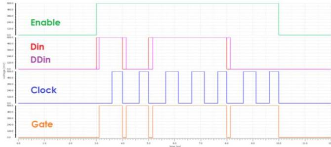
Fig. 9. Simulation results: Enable (green trace) triggers the GO that, starting from Din (red trace) first edge, generates the clock (Clock, blue trace). Clock samples DDin (violet trace) in the middle of the bit time, Gate (orange trace) resets Clock to 0 for any Din edge. In nominal conditions:  $\tau_{d,rise} = 163$   $\mu$ s,  $\tau_{d,fall} = 146$   $\mu$ s,  $\tau_{d,res} = 340$  ns.
