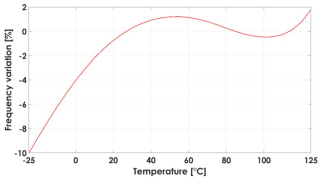
Fig. 12. Clock frequency variation with temperature.
