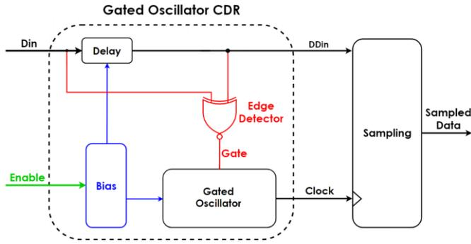
Fig. 3. Gated oscillator CDR circuit.
