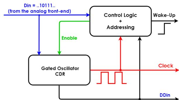
Fig. 2-A. Baseband logic. Din is the input data coming from the AFE, DDin is the delayed version of Din, Enable is used to turn on/off the CDR circuit.
