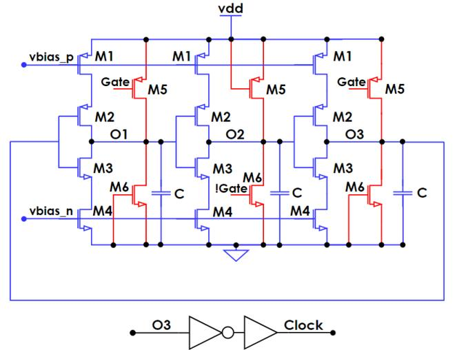
Fig. 6. Schematic of the proposed Gated Oscillator (GO).
