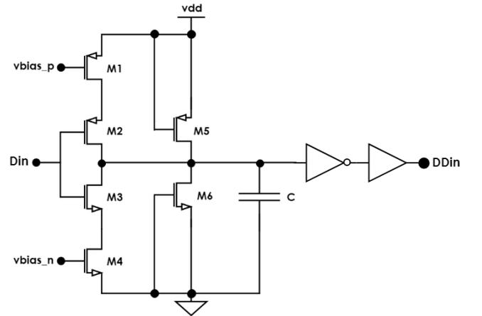
Figure 7. Schematic of the proposed Delay Block (DB).
