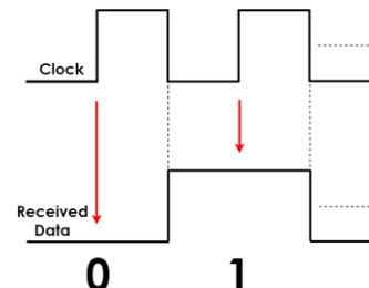
Fig. 2-B. Phase and frequency alignment between the received data and the clock signal generated by the CDR.
