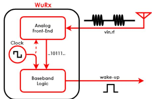
Fig. 1. Typical WuRx architecture. AFE may use or not an internal clock.
