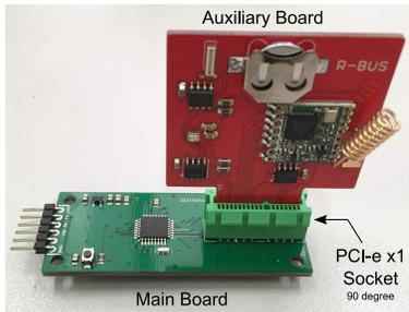
**Figure 1. R-Bus : Main and Auxiliary board Prototype**
