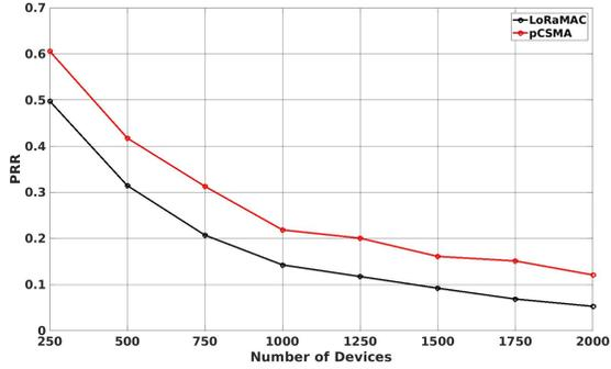
Figure 1: Packet Reception Ratio for increasing number of nodes for different MAC protocols - LoRaMAC (Aloha-like) and  $p$ -CSMA based with  $p = \frac{1}{N}$ . The devices transmit packets of 20 B periodically at 868.1 MHz using SF10.
