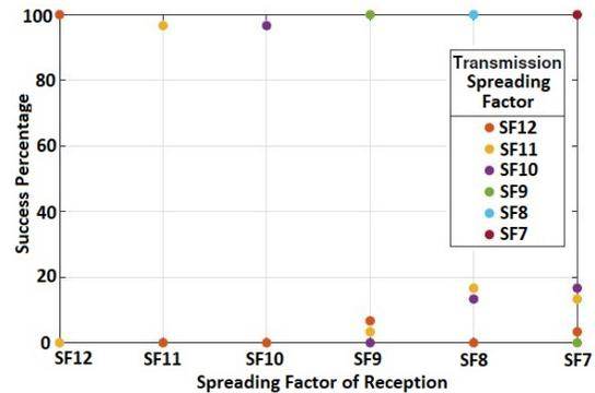
Figure 3: Success percentage of CAD when detecting preambles. The figure also shows the detection percentage across SFs; e.g., when the receiver was listening on SF7 it could also detect SF10 with  $\approx 19\%$  success.
