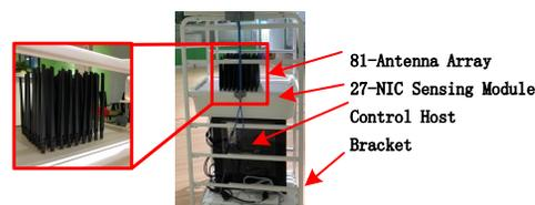
Figure 2. 81-antenna array controlled by PicoScenes
