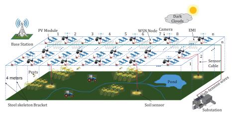
Figure 2. An ecosystem example of smart farming with Photovoltaic Agricultural Internet of Things.
