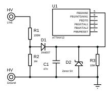
Figure 3: Schematic of the pulse detector. Neon bulbs are used to drop the high-voltage of the fence pulses to a manageable level which can be detected by an ADC converter in a low-power MCU.
