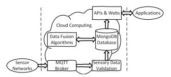
Figure 1: System architecture of the cloud-based services.
