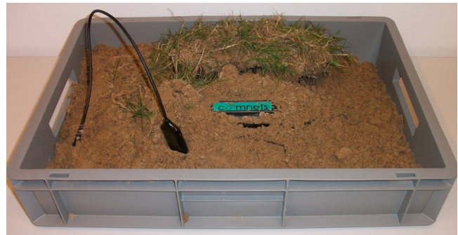
Figure 1. Application demo: Sensor and node placed in soil
