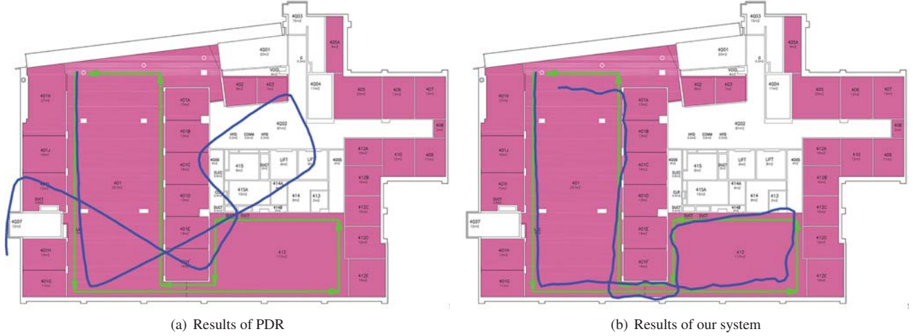
Figure 8: Experiments in lab, showing ground truth (green), results from PDR and NaviGlass (Best view in colour)
