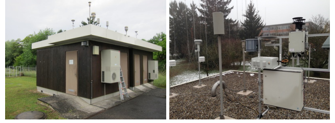
(a) NABEL air quality measurement station. (b) Air-inlets of the NABEL measurement station and our sensor testing box.
