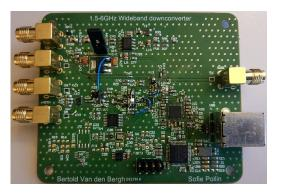
Figure 1. Prototype of the down-converter board
