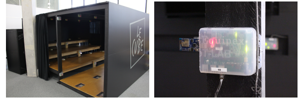
(a) Overall view (b) A TelosB connected Figure 2. Le Cube, an heterogeneous deployment of 64 open Gateways for interoperability testing.
