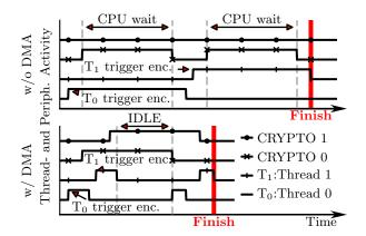
Figure 6. Qualitative comparison of thread and cryptoperipheral activity with (bottom) and without (top) CPU offloading using DMA.
