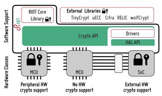
Figure 1. The software support layer of RIOT integrating crypto-peripherals, external crypto-devices, and crypto-libraries using a common crypto API.
