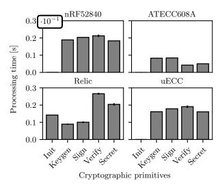
Figure 4. Processing time of different elliptic curve algorithms. Crypto-operations are either accelerated in hardware on the microcontroller (nRF52840), on an external chip (ATECC608A), or in software (Relic, uECC).
