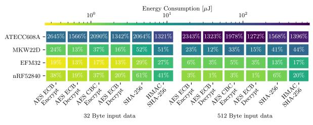
Figure 3. Energy consumption of hardware accelerated cryptographic operations on different platforms. Percentages show relative overhead compared to crypto-implementations in software running on the same devices.
