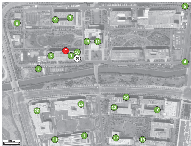
Figure 7. ChirpBox test installation in a University campus with twenty target nodes (green) and one control node (red). The white circle marks the location of a LoRaWAN gateway.
