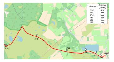
Figure 5: A map indicating the route taken (red line) and the sensing ranges for different SFs. The receivers were stationary (indicated by the point 'SENSOR' in the figure) and the transmitter was on a bicycle. The calculated ranges are the straight-line distances (not the distance the bicycle traversed).
