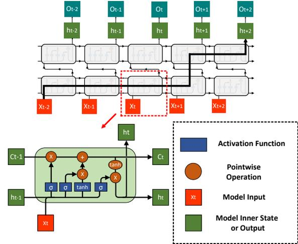
Figure 3. LSTM network structure
