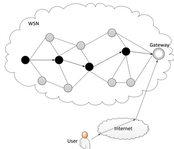
Figure 1. Structure of Wireless Sensor Network
