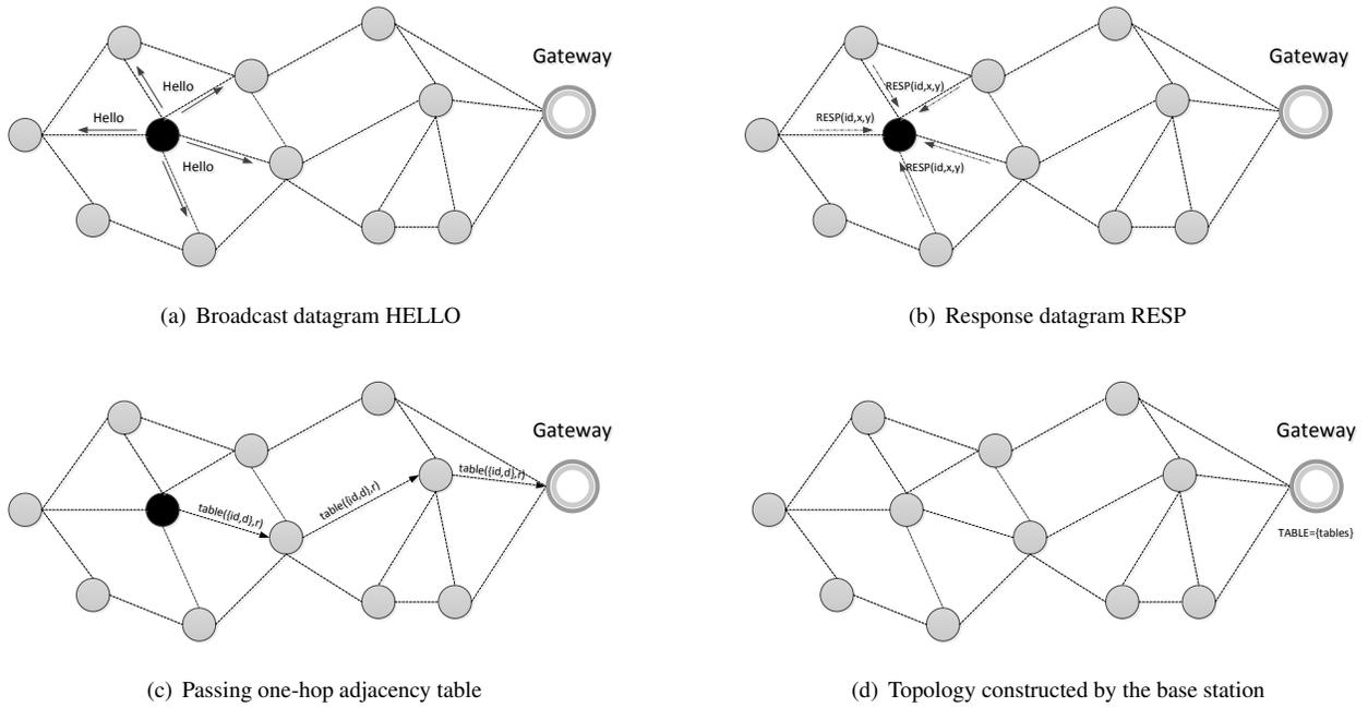
**Figure 3. Illustration of Construction Process for Topological Model**
