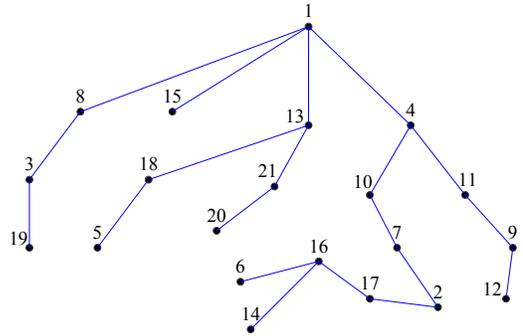
Figure 6. Topological Structure of Network Constructed by RPL
