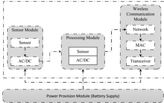
**Figure 2. Structure of Wireless Sensor Network**
