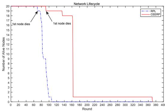
**Figure 8. Rounds in Which the First Sensor Node Dies**
