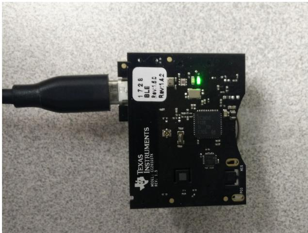
Figure 9. Programming CC2650STK SensorTag
