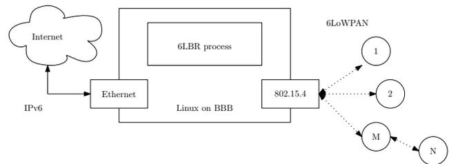
Figure 3. Border router block diagram
