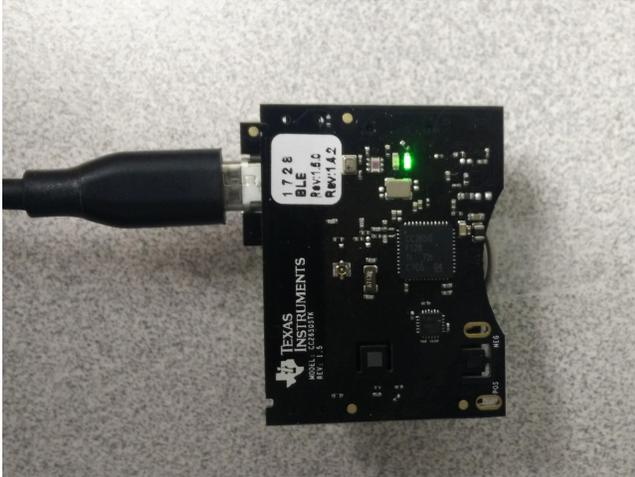
Figure 9. Programming CC2650STK SensorTag
