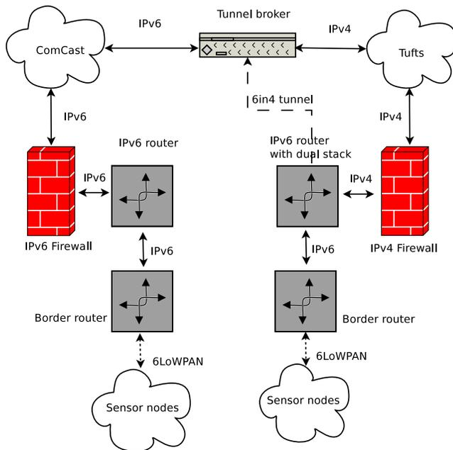
Figure 7. 6LoWPAN platform testbed
