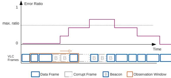
Figure 5. Simplified example of the error ratio method.
