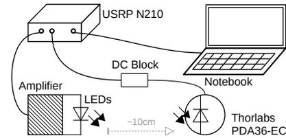
Figure 2. Measurement lab setup.
