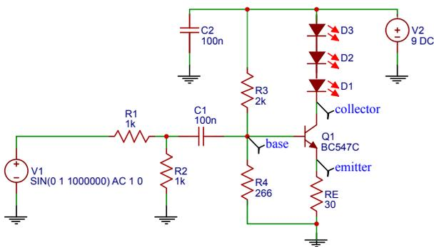
Figure 1. Schematic of our low-cost transmitter front-end.
