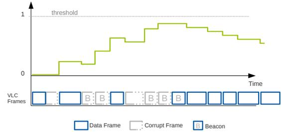
Figure 6. Example of a simple threshold decision algorithm.
