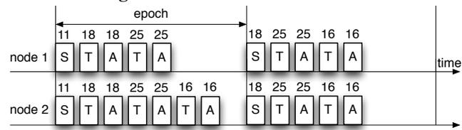
Figure 2. Channel hopping in CRYSTAL.
