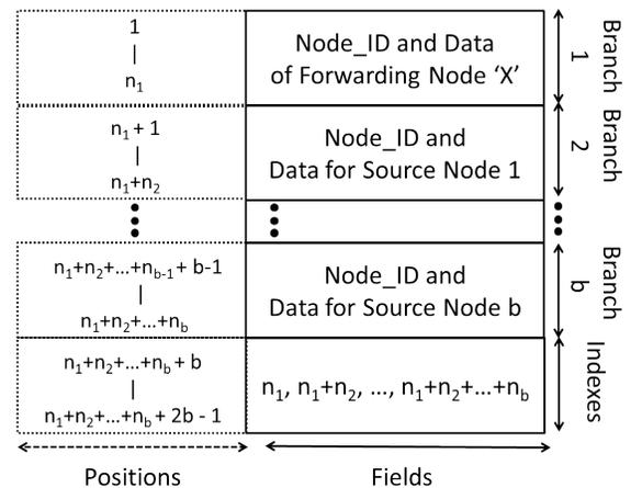
Figure 1. Data Structure used in the R2EDC Protocol.
