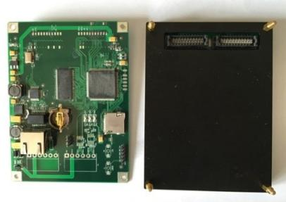
Figure 2. Digital signal processing board and radio frequency detection part of the prototype.
