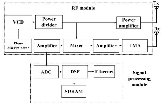
**Figure 4. Architecture design overview of our FMCW radar prototype**
