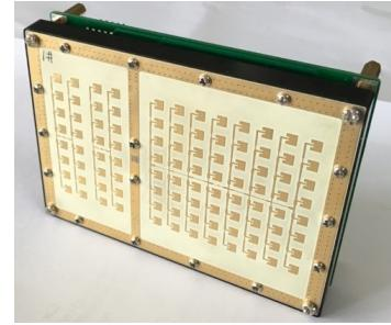
Figure 1. 24GHz FMCW radar prototype with 1Tx and 2Rx antenna arrays.
