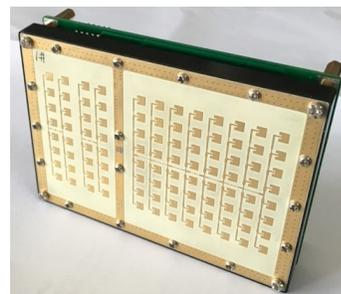
Figure 1. 24GHz FMCW radar prototype with 1Tx and 2Rx antenna arrays.
