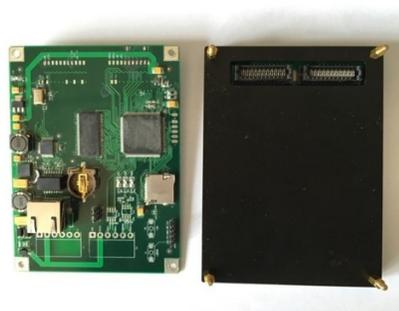
Figure 2. Digital signal processing board and radio frequency detection part of the prototype.
