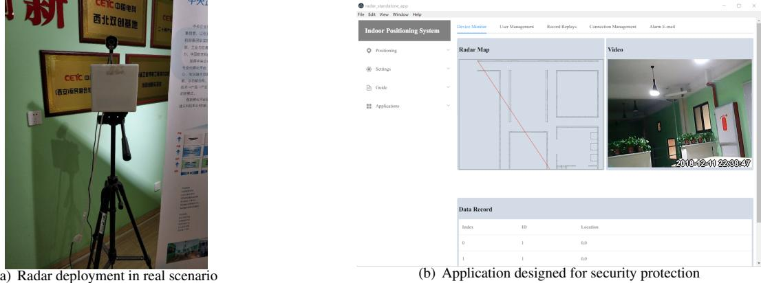
**Figure 3.** Experimental Setup with our prototype, and it is a packaged device with wave-transmitting material. We develop and implement a tailored software to show the real-time positioning status of multi-targets.
