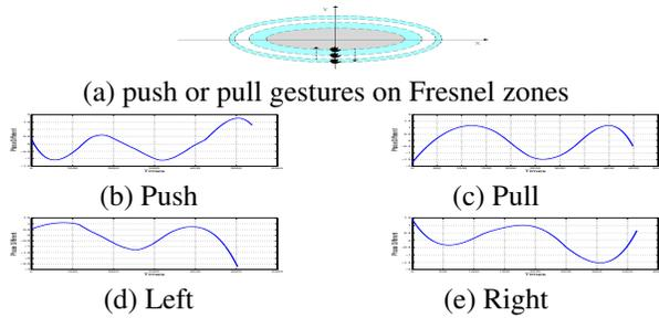
Figure 2: Phase difference waveform of push and pull gestures
