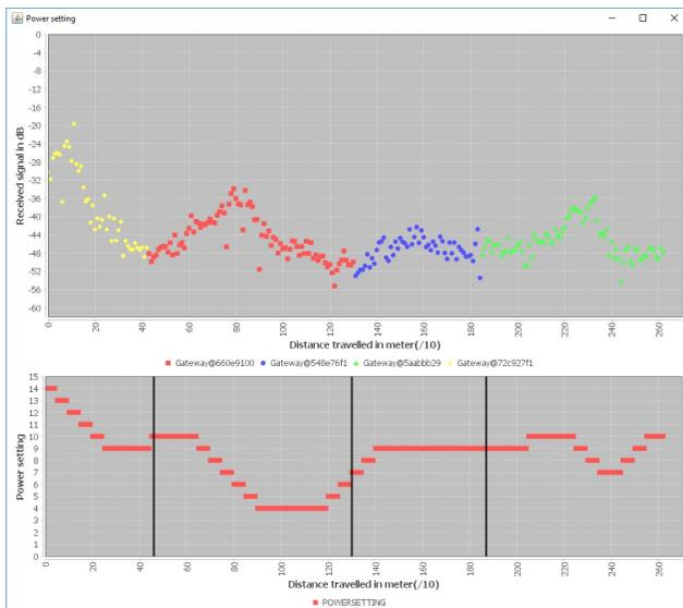
Figure 2. Signals received from D1 and power adaptation
