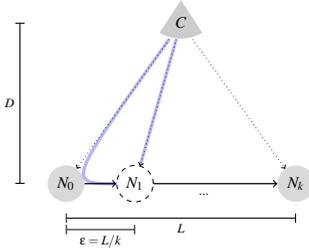
**Figure 1. Single-hop and multi-hop scenarios with a single carrier generator (C). Carrier-assisted devices ( $N_0 \dots N_k$ ) are arranged on a regular linear grid of  $k+1$  nodes covering the distance  $L$ .**
