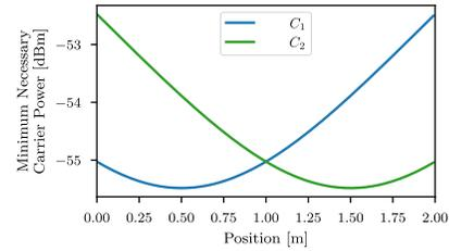
**Figure 4. The carrier generator requires minimum power when it is aligned with the carrier-assisted node. The further the distance, higher the power required. After a threshold the carrier source can be transferred to another carrier generator to reduce the necessary power.**
