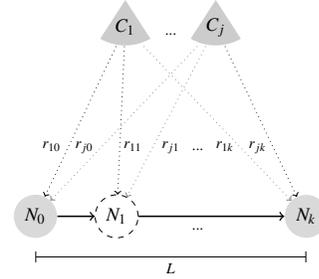
**Figure 3. Multiple carrier generators providing carrier for multiple carrier-assisted devices. Messages are relayed by  $k$  nodes to traverse the distance  $L$ .**
