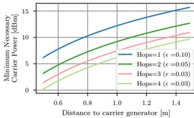
**Figure 2. Minimum Carrier Power required for Multiple Hops. As the carrier generator moves away from the nodes, the necessary output power increases. Increasing the number of hops decreases the distance offsets the necessary carrier output power.**
