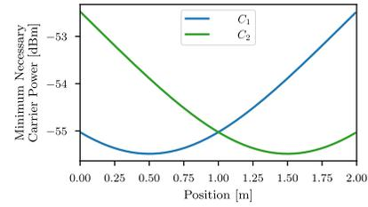
**Figure 4. The carrier generator requires minimum power when it is aligned with the carrier-assisted node. The further the distance, higher the power required. After a threshold the carrier source can be transferred to another carrier generator to reduce the necessary power.**
