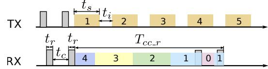
Figure 1. The duration of  $N_s = n$  ( $0 \leq n \leq N_{max}$ ) as the start sending position varies in  $T_{cc,r}$  of the receiver.
