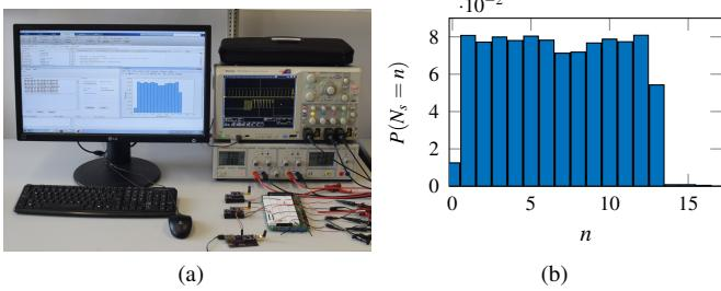
**Figure 2.** a) Experiment setup. b) The measured PMF of  $N_s$  when the receiver’s CCR is 32 Hz with 2 hours of data.
