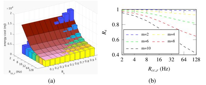
**Figure 3.** a). The overall average energy cost with and without using event-triggered state estimation; b) The transmission rate boundary to ensure energy saving.
