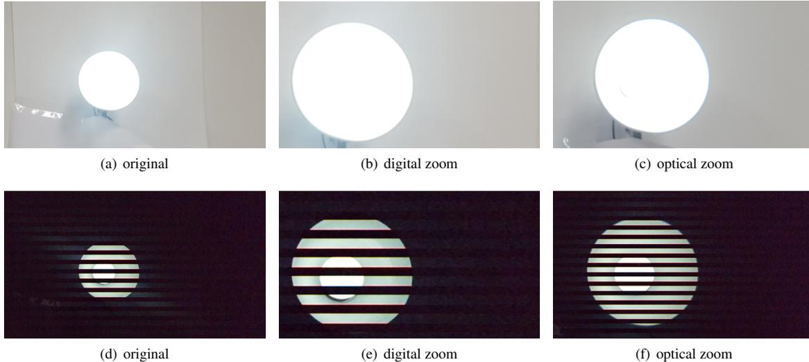
Figure 2: This shows that the optical zoom differs in the number of bands, although the height size in pixels is the same. Figures 2(a)-(c) are taken with long exposure time, and both zooms magnify the light two-fold. But in Figures 2(d)-(f), taken with short exposure time, the digital zoom magnifies the band itself, while the optical zoom captures twice the bands.
