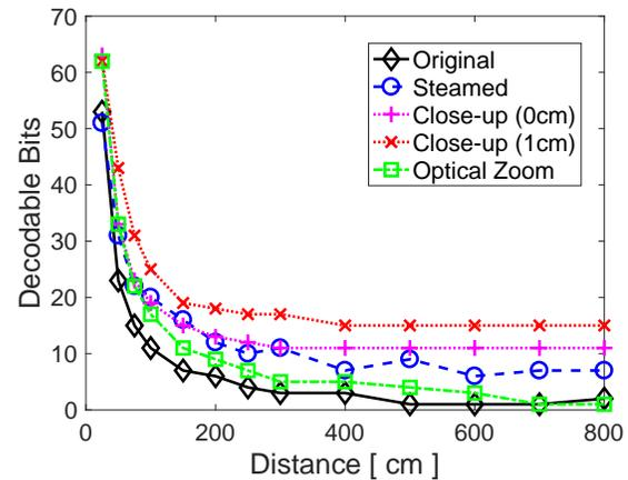
Figure 5: Decoded bits of various filters by distance.
