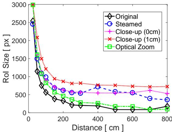
Figure 4: ROI size comparison of various filters by distance.
