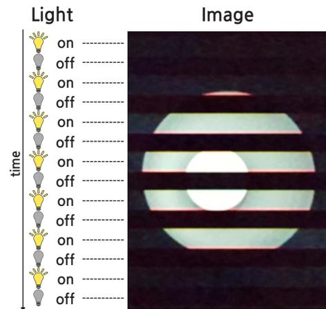
Figure 1: This figure shows the basic mechanism of the rolling shutter camera. The left side of the figure shows the light's on/off status while time goes by. The right side is the resultant image taken by the camera image sensor, in which the rolling shutter works row-by-row.
