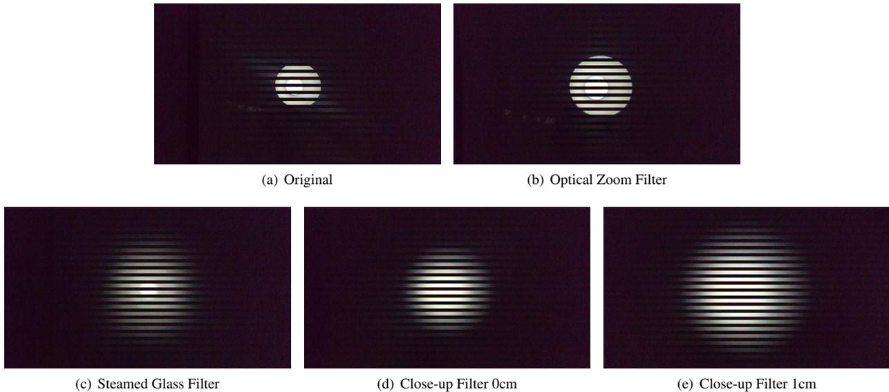
Figure 3: Comparison of the images taken with various filters. The images are all taken at the same distance of 100 cm. In Figure 3(e), we fitted the close-up filter 1 cm away from the camera.
