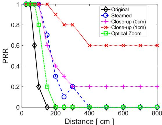
Figure 6: Packet Reception Rate comparison of various filters by distance.
