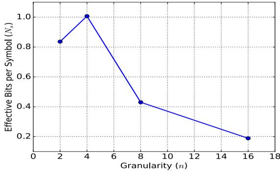
Figure 6: Channel Performance for RSSI Based Location Signaling Using Parity Bit Channel Coding and Real Measurements
