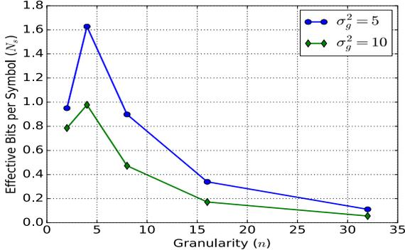
Figure 3: Performance of LOCO Using Parity Bit Channel Coding under Gaussian Noise Model
