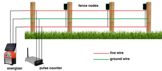
Figure 1: Components of the elephant electric fence breakage detection system. The *energizer* generates a series of high-voltage pulses at a constant rate which are randomly grounded by *fence nodes*. The *pulse counter* identifies the absence of pulses.
