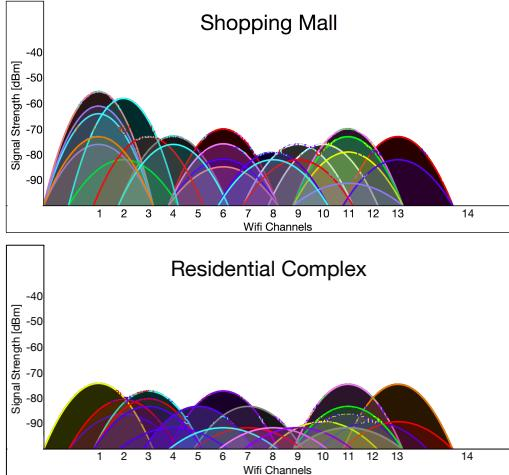
**Figure 2. Severe interference due to unplanned-CTI.**
