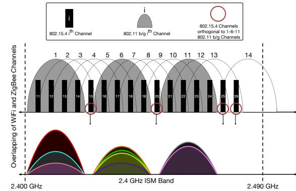
**Figure 1. Coexistence of ZigBee and WiFi in the 2.4GHz ISM band having planned-CTI. WiFi scan illustration from inside an academic institute.**
