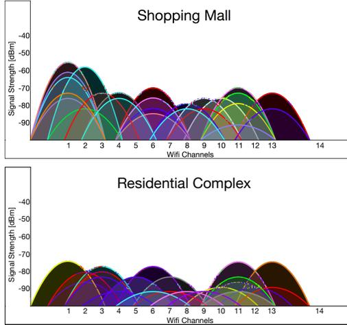
Figure 2. Severe interference due to unplanned-CTI.
