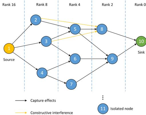
Figure 1. Oriented flooding avoids isolated node problem.
