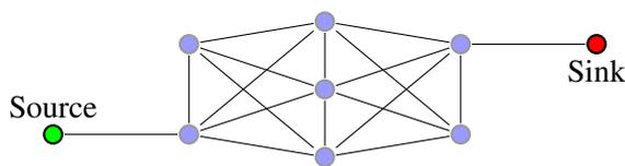
Figure 2: Multi-hop set-up: 2 devices will communicate with each other in a multi-hop fashion using the nodes in the middle.
