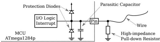
**Figure 2. Circuit for Pulse Detection**
