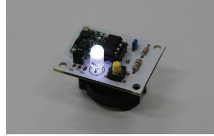
**Figure 4. Temperature measurement board.** It consists of ATtiny85 as a microcomputer, a 5 mm LED, a temperature sensor, a tact switch, and a power circuit.
