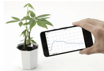
Figure 2. A LED-to-camera communication example. This communication enables easy visualization of the data stored in sensing devices.
