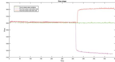
Figure 4. Flow shapes before and after leak
