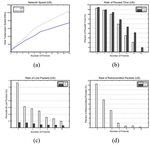
Figure 2. (a)Relation between number of fog nodes and network speed (b)(c)(d)Experiment results of TCP/UDP implementation
