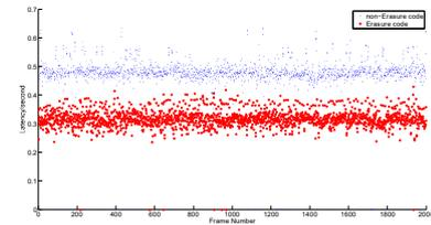
Figure 3. Latency of Transmission Model Based on Erasure Code and that of Traditional Model
