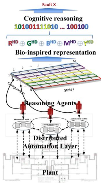
**Figure 1. Distributed fault detection system empowered by vector symbolic architectures. Tested for generic nuclear power plant model [7].**
