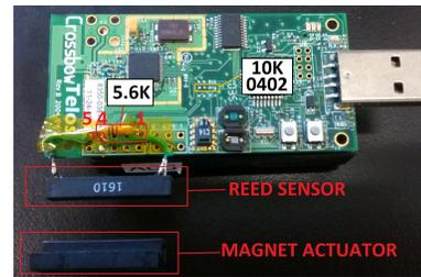
Figure 2. Wireless Sensor for Zone Monitoring
