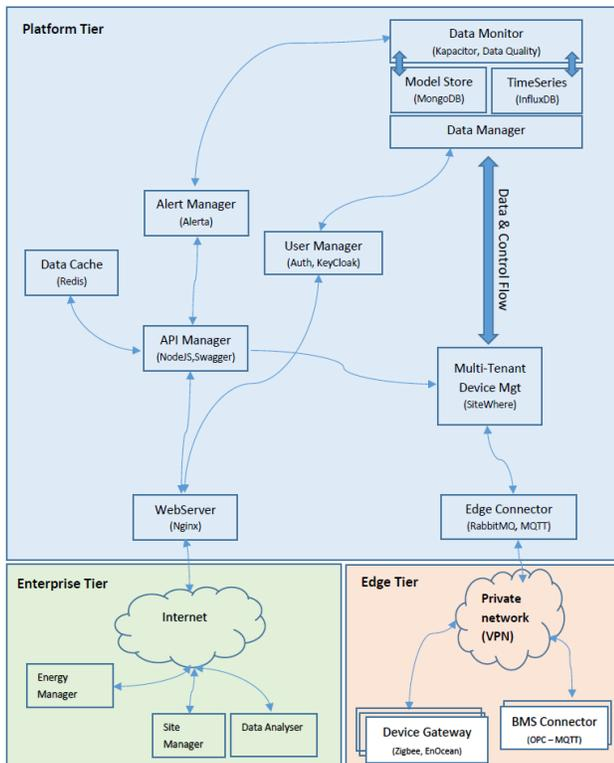
Figure 1. R4Platform three Tier Architecture
