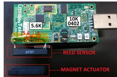
Figure 2. Wireless Sensor for Zone Monitoring
