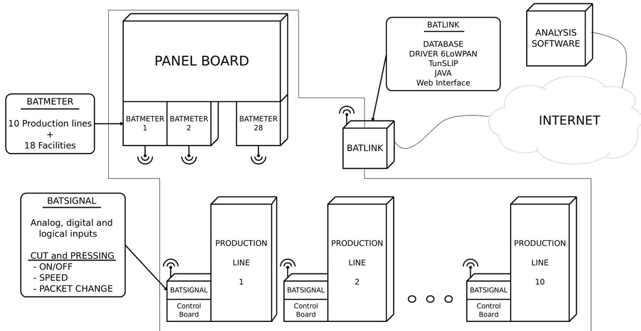
Figure 2. Solution architecture.
