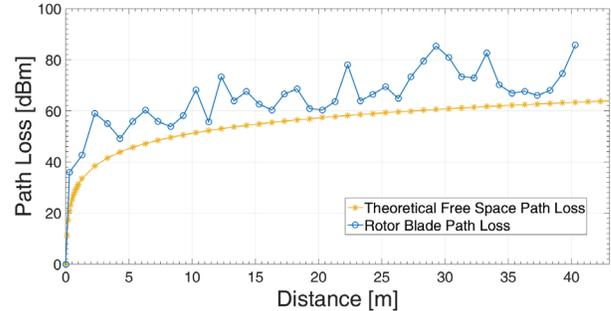
Figure 3. Path Loss Comparison 868 Mhz
