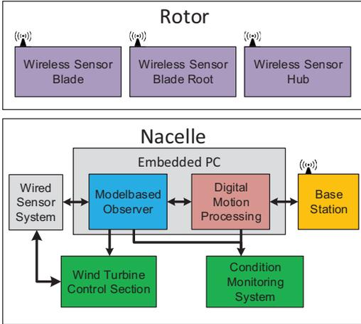
Figure 2. Topology of the Wireless Sensor System
