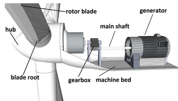
Figure 1. Wind turbine drive train consisting of generator, main shaft, gearbox and rotor
